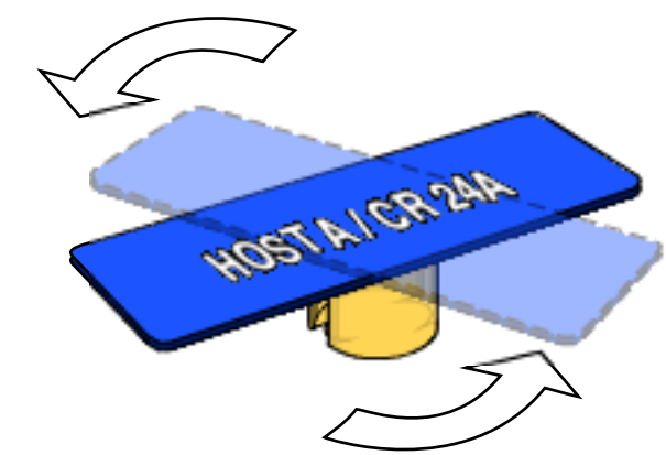
6 WRITING SURFACE 360° ROTATION EITHER METHOD WILL ALLOW FOR ROTATION OF WRITING SURFACE
