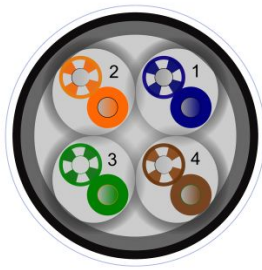
Figure 1. UTP (Unshielded Twisted Pair) cross-section.
